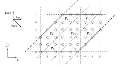
For this problem, optimal transformation methods for systolic arrays produce matrices:
